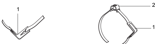
Fig. 6.43: Tension strap with metal spring and clamp
