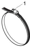
Fig. 6.25: Tension strap with band clamp clasp
