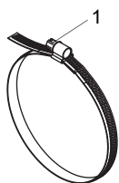
Fig. 6.49: Tension strap with band clamp clasp
